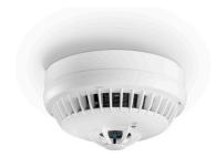
Intelligent optical and thermal multi sensor detector for loop3000 with two optical and two thermal sensors and a bidirectional isolator for earliest fire detection and indication in all environments with difficult ambient conditions, according to EN 54-5/-7 /-17, prEN 54-29 and CEA 4021. Fusion® technology for the detection of the smallest smoke particles and fires in the early stage by using the wavelengths of the wide-band white light spectrum.
